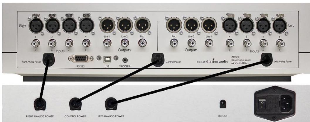
The Altair II's separate power supply (bottom component in the picture above) must be connected to the Altair II main chassis (top component in the picture above) as shown above before you plug the unit into a wall. Make sure the power switch on the power supply is in the off (O) position.
