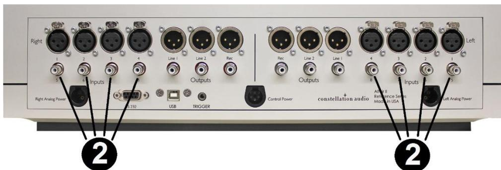
These unbalanced inputs are provided as a convenience for use with unbalanced signal sources. Whenever possible, we recommend using XLR connections instead. Connecting to an unbalanced source is handled in the same way an XLR balanced source.
