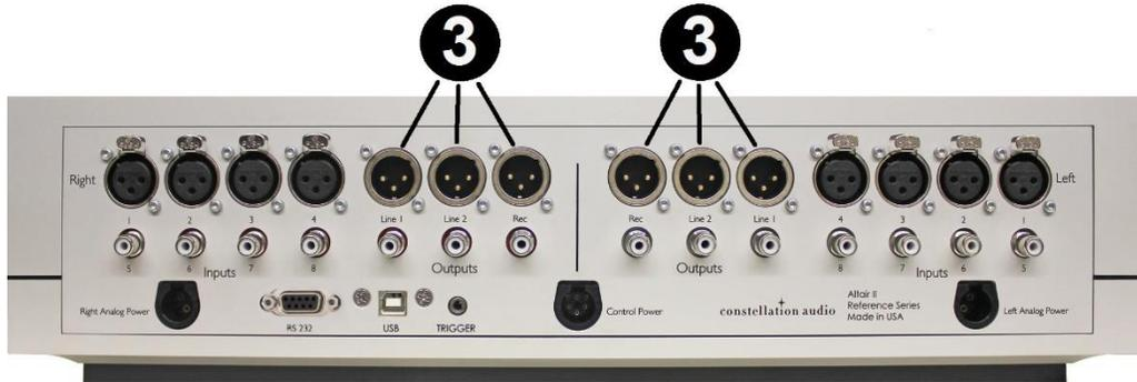
The inner six XLR connections on the rear of the Altair II are outputs. The signal at these outputs is the same—it does not matter if you use output 1 or output 2. To remove an XLR plug, push on the tab on the connector body and pull the plug out.
