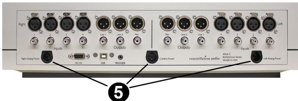
These inputs connect to the power outputs of the Altair II's separate power supply. The Altair II includes special spiral-wrapped, gold-plated copper cables designed for aerospace use. Each cable is rated to handle 30 amps.
