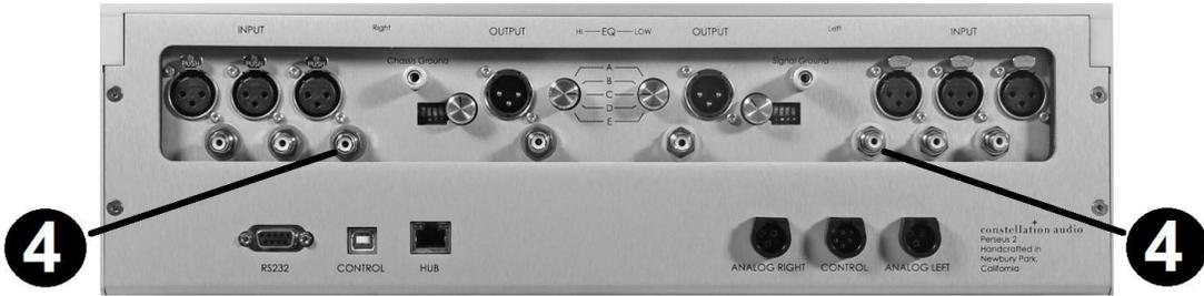
This unbalanced input is provided as a convenience for use with turntables having only unbalanced output. Whenever possible, we recommend using XLR connections instead. Connecting to an unbalanced source is handled in the same way an XLR balanced source.
