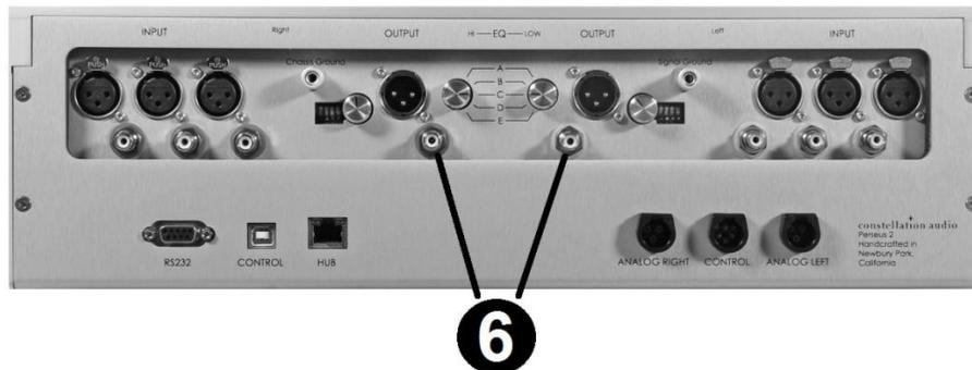
RCA unbalanced outputs are also supplied for preamplifiers not equipped with XLR connections. When connecting to an amplifier, be sure to match the output to the correct channel on your amp. As you are looking at the back of the Perseus, the output on the left side is for the right channel, and the output on the right is for the left channel. To remove an RCA plug, grasp it by the connector body and pull the plug out.
