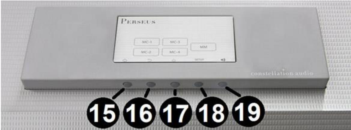
The front panel includes an LCD touchscreen and five buttons positioned underneath the display. These buttons work along with the touchscreen to provide control and monitoring of most Perseus functions. The functions of the buttons are shown using icons on the screen. Here are the functions:
