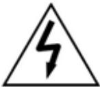
The lightning flash with arrowhead, within an equilateral triangle, is intended to alert the user to the presence of uninsulated dangerous voltage within the product enclosure that may be of sufficient magnitude to constitute a risk of electrical shock to persons.
