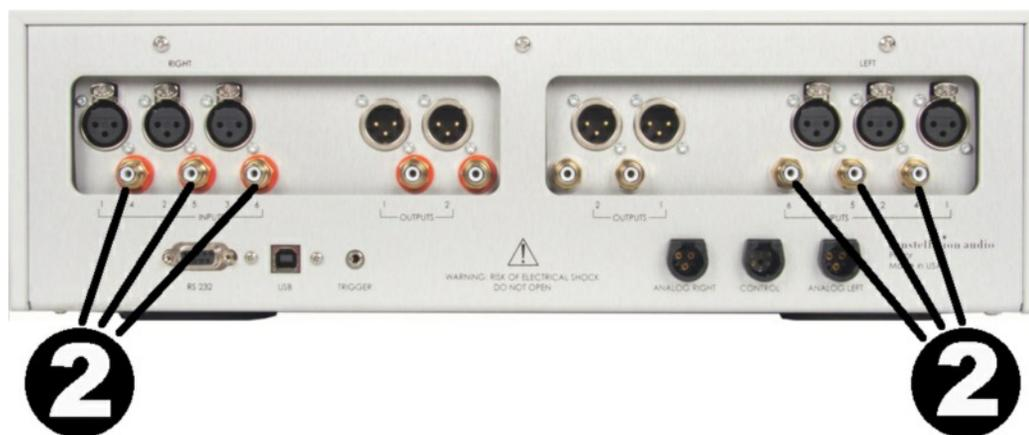
These unbalanced inputs are provided as a convenience for use with unbalanced signal sources. Whenever possible, we recommend using XLR connections instead. Connecting to an unbalanced source is handled in the same way an XLR balanced source. To remove an RCA plug, grasp the plug and pull it out. Do not pull on the cable.
