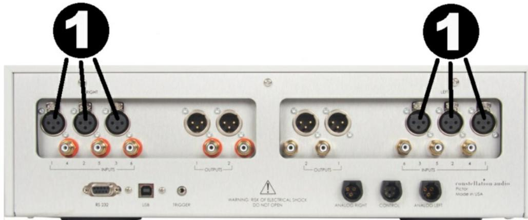
On the rear of the Pictor are six XLR inputs, two on each side. As you are looking at the rear panel, the left three XLR inputs are for the right channel, the right three inputs are for the left channel. Underneath each jack is the corresponding input number. Use of XLR connections is recommended for the best possible audio quality. To remove an XLR plug, push on the tab above the jack and pull the plug out.
