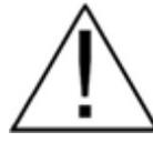
The exclamation point within an equilateral triangle is intended to alert the user to the presence of important operating maintenance (servicing) instructions in the literature accompanying the appliance.
