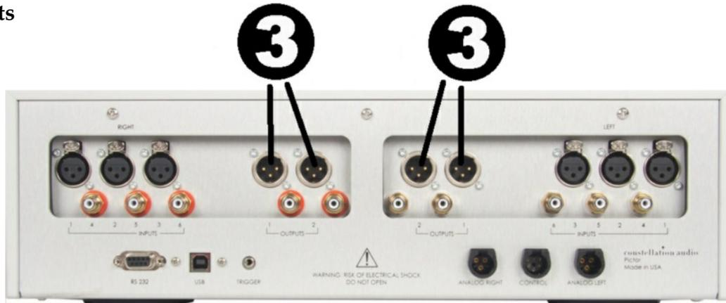
The inner XLR connections on the rear of the Pictor are outputs. The signal at these outputs is the same—it does not matter if you use output 1 or output 2. To remove an XLR plug, push on the tab on the connector body and pull the plug out.
