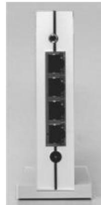
For best results, place the Pulsar RF hub away from metal objects. Range of the Pulsar RF hub is up to 50 feet, but this range may be affected by the position and orientation of the hub. If the Pyxis remote works reliably, there is no need to be concerned about the range. If you experience inconsistent operation—i.e., if pushing a button on the Pyxis sometimes doesn't cause the components to respond—try turning the Pulsar RF hub in another direction or moving it to a different location.
