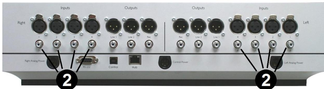
These unbalanced inputs are provided as a convenience for use with unbalanced signal sources. Whenever possible, we recommend using XLR connections instead. Connecting to an unbalanced source is handled in the same way an XLR balanced source.
