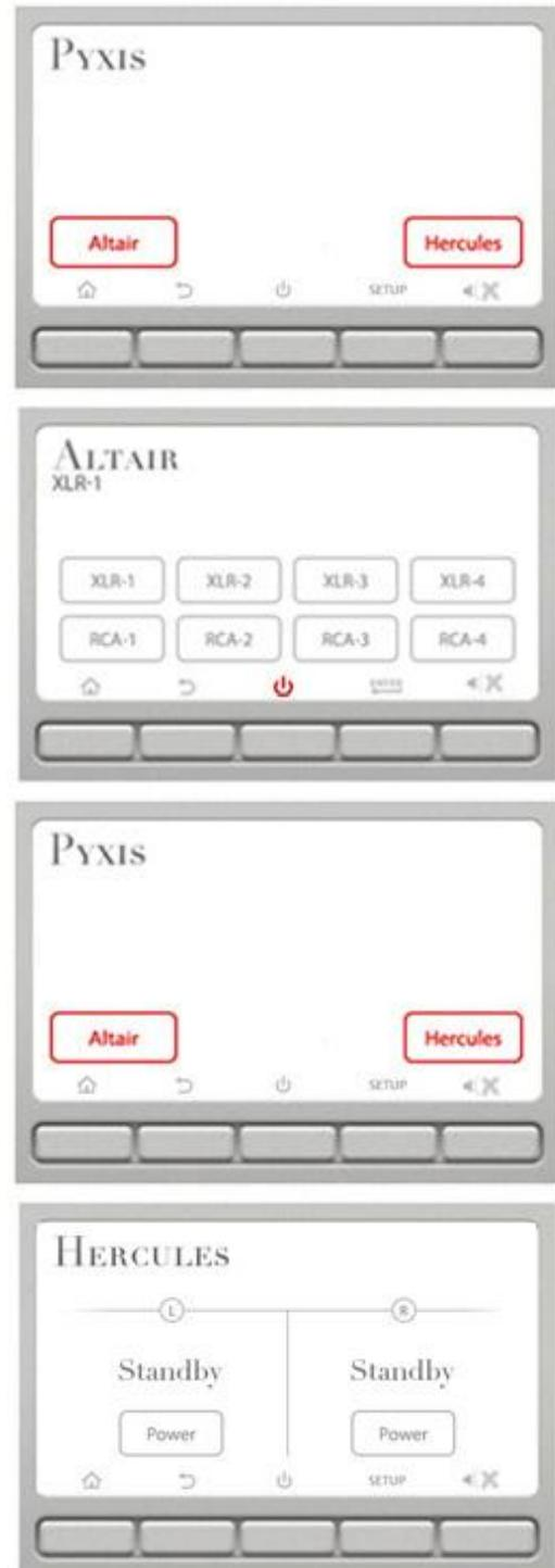
The components will go through a warm-up cycle lasting 1 minute. At the end of this cycle the onscreen buttons for the components should turn blue. If the Hercules button instead turns yellow, either one of the Hercules amplifiers has not been switched on or its AC power has been disconnected. To correct the problem, return to the Hercules power screen by tapping the onscreen Hercules button.
