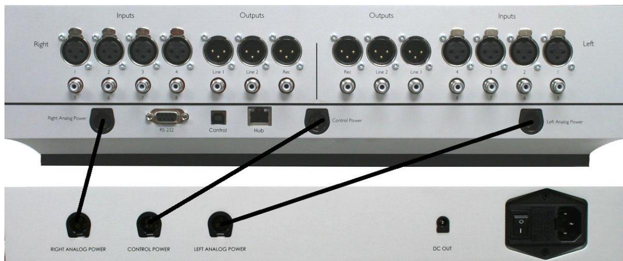
The Altair's separate power supply (bottom) must be connected to the Altair (top) as shown above before you plug the unit into a wall. Make sure the power switch (right) on the power supply is in the off (O) position.
