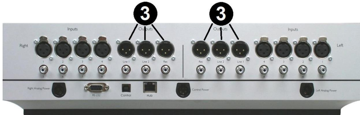
The inner six XLR connections on the rear of the Altair are outputs. The outer four of these are for connection to amplifiers, while the inner two are fixed-level outputs for connection to a recording device. To remove an XLR plug, push on the tab on the connector body and pull the plug out.
