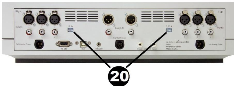
These two arrays of four microswitches each adjust loading for the MM input. You can flick the switches gently with a small screwdriver, a toothpick, etc. Up is on, down is off. Use the settings recommended by the manufacturer of your cartridge, or experiment and use the settings that sound best to you. But always use the same settings on both switch arrays. Below are the functions for each switch:
