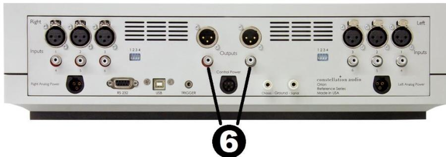
RCA unbalanced outputs are also supplied for preamplifiers not equipped with XLR connections. When connecting to an amplifier, be sure to match the output to the correct channel on your amp. As you are looking at the back of the Orion, the output on the left side is for the right channel, and the output on the right is for the left channel. To remove an RCA plug, grasp it by the connector body and pull the plug out.
