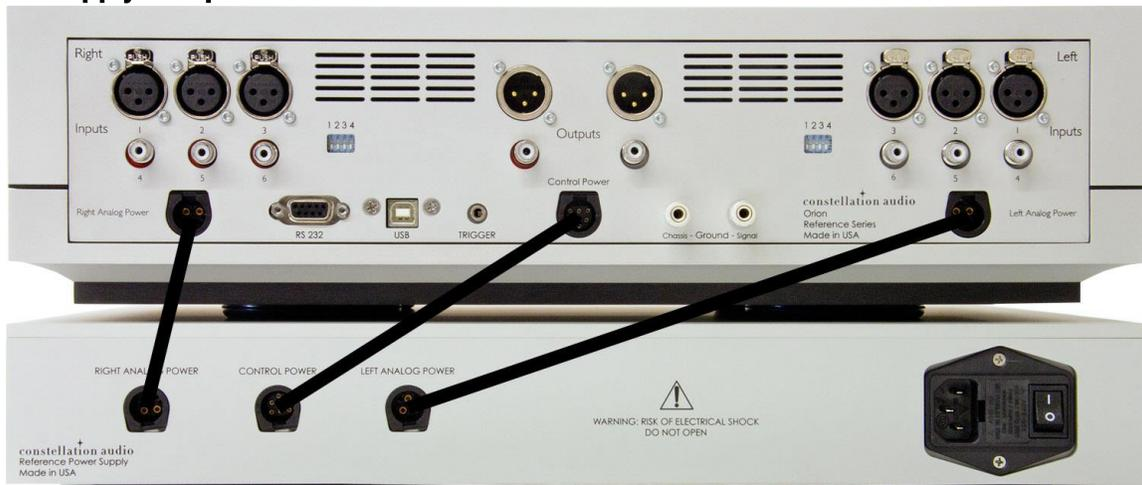
The Orion's separate power supply (bottom component in the picture above) must be connected to the Orion main chassis (top component in the picture above) as shown above before you plug the unit into a wall. Make sure the power switch on the power supply is in the off (O) position.
