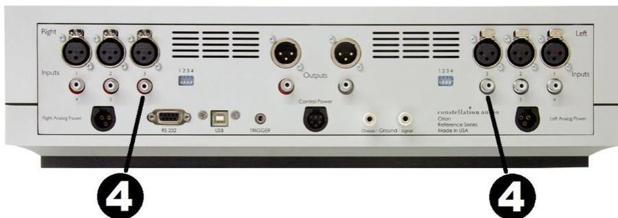
This unbalanced input is provided as a convenience for use with turntables having only unbalanced output. Whenever possible, we recommend using XLR connections instead. Connecting to an unbalanced source is handled in the same way an XLR balanced source.
