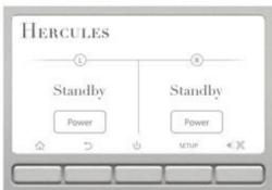
The components will go through a warm-up cycle lasting 1 minute. At the end of this cycle the onscreen buttons for the components should turn blue. If the Hercules button instead turns yellow, either one of the Hercules amplifiers has not been switched on or its AC power has been disconnected. To correct the problem, return to the Hercules power screen by tapping the onscreen Hercules button.
