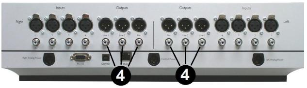
RCA unbalanced outputs are also supplied for amplifiers not equipped with XLR connections. The outer four of these are for connection to amplifiers, while the inner two are fixed-level outputs for connection to a recording device.
