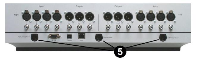
These inputs connect to the power outputs of the Altair's separate power supply. Constellation Audio has supplied you with special spiral-wrapped, gold-plated copper cables designed for aerospace use. Each of these cables is rated to handle 30 amps.
