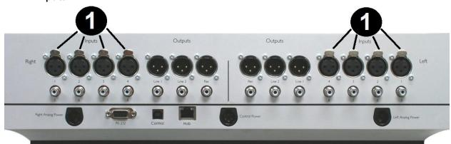
On the rear of the Altair preamp there are eight XLR inputs, four on each side. As you are looking at the rear panel, the left four XLR inputs are for the right channel, the right four inputs are for the left channel. Underneath each jack is the corresponding input number. Use of XLR connections is recommended for the best possible audio quality. To remove an XLR plug, push on the tab above the jack and pull the plug out.
