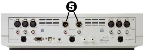
The inner XLR connections on the rear of the Orion are outputs. To remove an XLR plug, push on the tab on the connector body and pull the plug out. Be sure to match the output to the correct channel on your preamp. As you are looking at the back of the Orion, the output on the left side is for the right channel, the output on the right is for the left channel.
