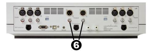
RCA unbalanced outputs are also supplied for preamplifers not equipped with XLR connections. When connecting to an amplifier, be sure to match the output to the correct channel on your amp. As you are looking at the back of the Orion, the output on the left side is for the right channel, and the output on the right is for the left channel. To remove an RCA plug, grasp it by the connector body and pull the plug out.
