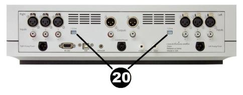
These two arrays of four microswitches each adjust loading for the MM input. You can flick the switches gently with a small screwdriver, a toothpick, etc. <u>Up is on, down is off.</u> Use the settings recommended by the manufacturer of your cartridge, or experiment and use the settings that sound best to you. But always use the same settings on both switch arrays. Below are the functions for each switch:
