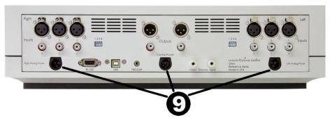
These inputs connect to the power outputs of the Orion's separate power supply. The Orion power supply includes permanently attached, spiral-wrapped, gold-plated copper cables designed for aerospace use. Each cable is rated to handle 30 amps.
