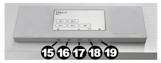
The front panel includes an LCD touchscreen and five buttons positioned underneath the display. These buttons work along with the touchscreen to provide control and monitoring of most Orion functions. The functions of the buttons are shown using icons on the screen. Here are the functions:
